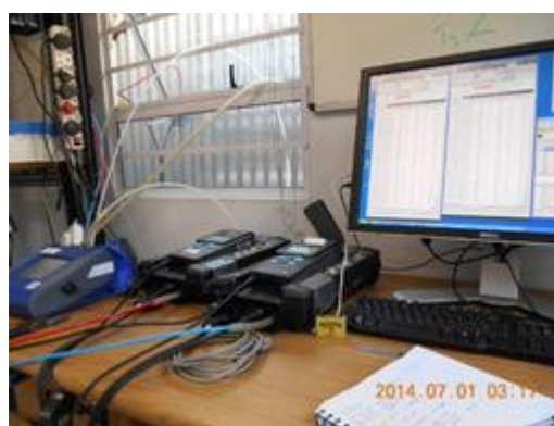
Fig 3. Flue gas analysers and data capturing equipment set-up at SeTAR stove testing lab.
