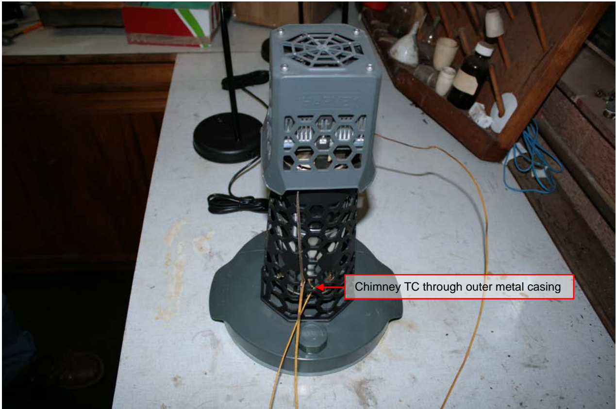
Figure 2.2.5: Chimney TC was placed through outer metal casing onto inner chimney pipe
