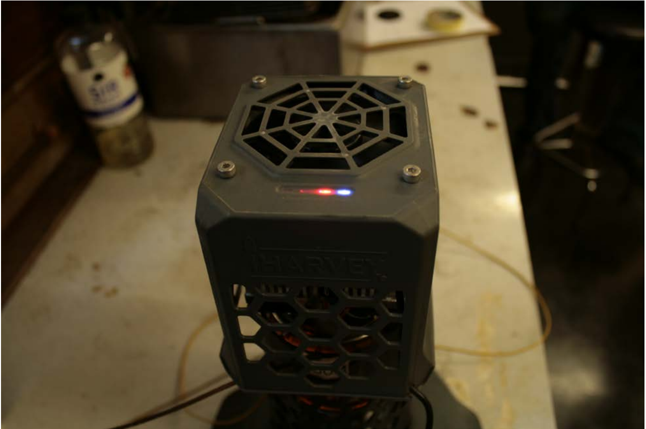
Figure 2.2.7: Red light; Excessive heat for power generation – Blue light; Excess power available
