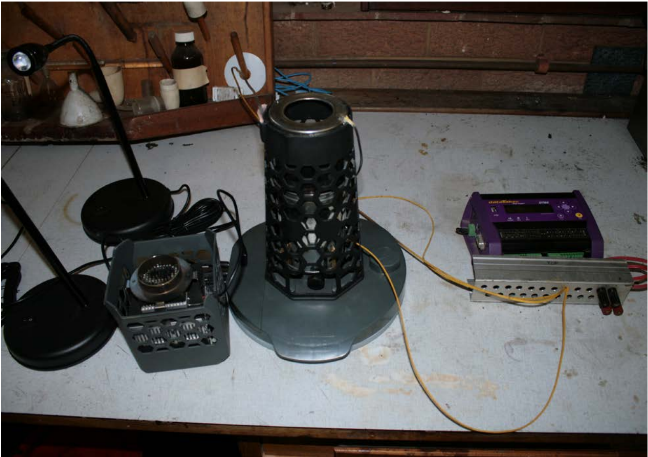
Figure 2.2.3: Test setup for iHarvey Power Generator with Data logger
