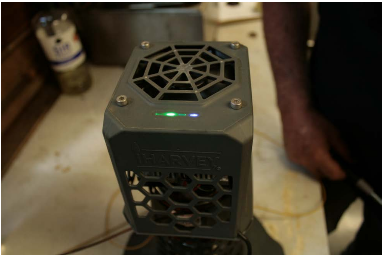
Figure 2.2.6: Green light; adequate heat for power generation – Blue light; Excess power available
